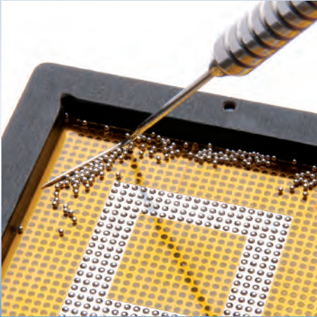
Filling solder spheres in the stencil holes.
