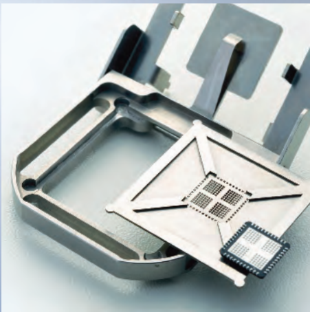
Installation of stencil into prebumping tool.
